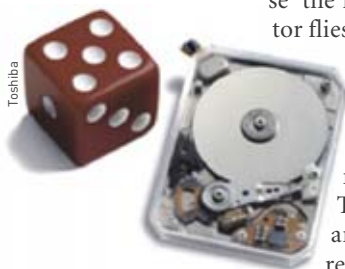
Figure 3. Disk made by Toshiba measuring 2 cm in diameter with a capacity of 4 GB and weighing a mere 8.5 g!
