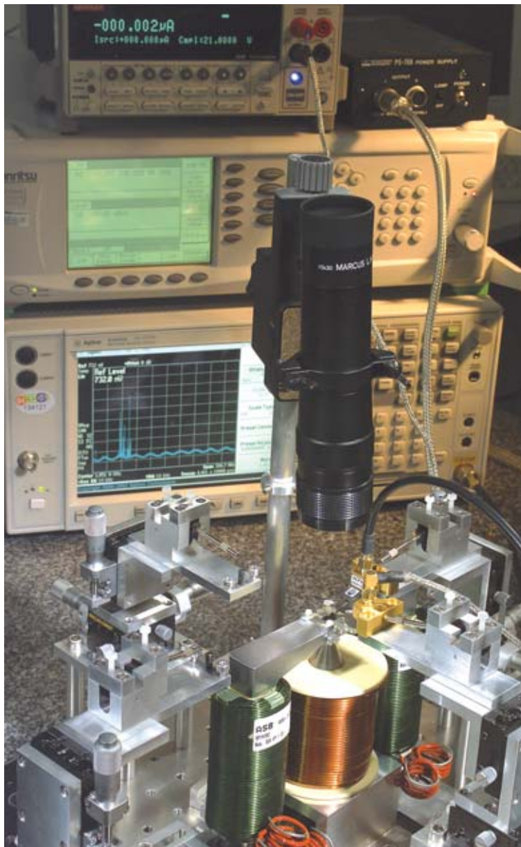
Instrumentation for broadband electrical spectral measurement (0–26 GHz) dedicated to the study of spin-polarised current magnetic nanostructures at CEA Grenoble.
