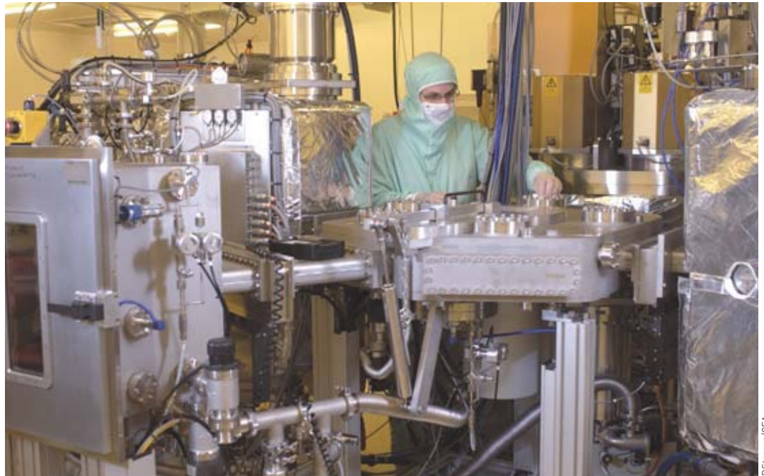
Magnetic thin layer deposition machine for the manufacture of MRAMs at CEA Grenoble.
